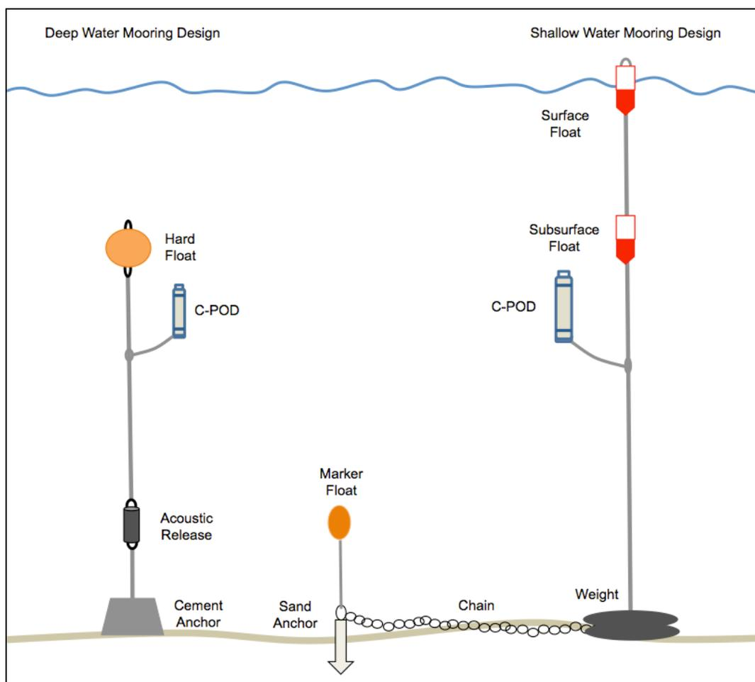
Schematic diagram of C-POD mooring designs (not to scale). Moorings at locations with water depths greater than 30 m were installed using the deep water (left) design, while Moorings at locations with water depths less than 30 m were installed using the shallow water (right) design. The shallow water design required scientific diver installation and retrieval, while the deep-water design required the use of acoustic releases.
